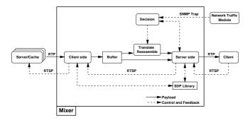
Figure 3. Internal architecture of our mixer.
