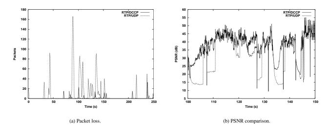
Figure 6. Packet loss and PSNR comparison results.
